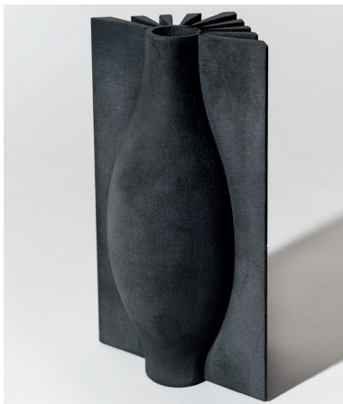
Fig. 3 Prototype in generative shaping made of RBSiC by Schunk Ingenieurkeramik GmbH (Source: Raisa Galofre MA, Berlin)
