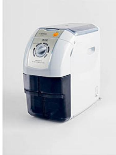
Used in Japan to remove the endocarp (outer layer) of rice by whirring the grains against an abrasive surface, making it easier for koji to take hold. A grain polisher will work equally well with lesser-known grains, like emmer or konini.
