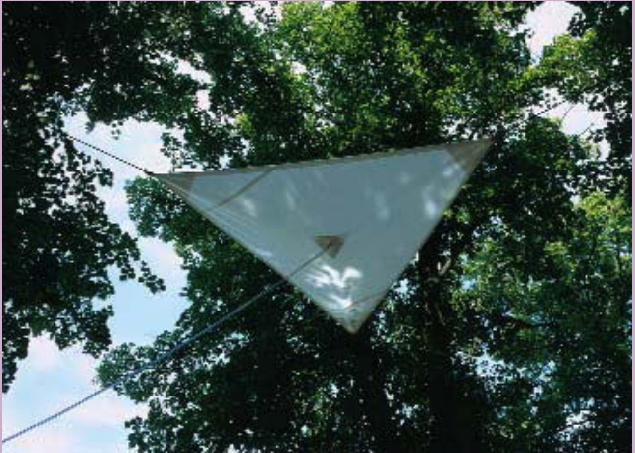
Water Collector: Acrylic sheet collects rain water. The water is directed to the water tanks through a hose.
