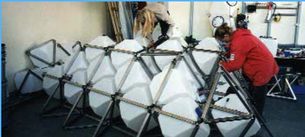
Assembling the FLOATING PLATFORM at FACTORY.
