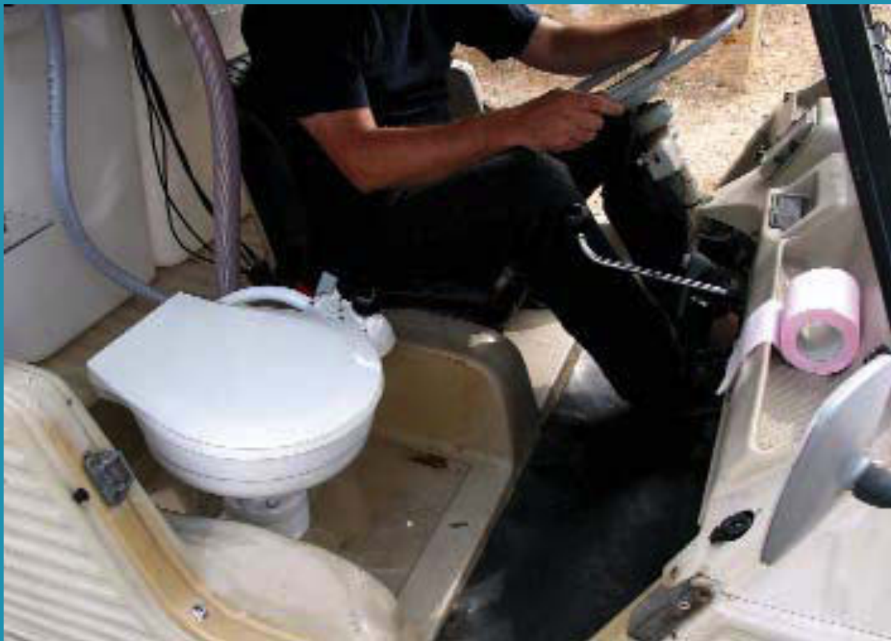
Toilet, mounted in place of the passenger seat (Méhari version)
