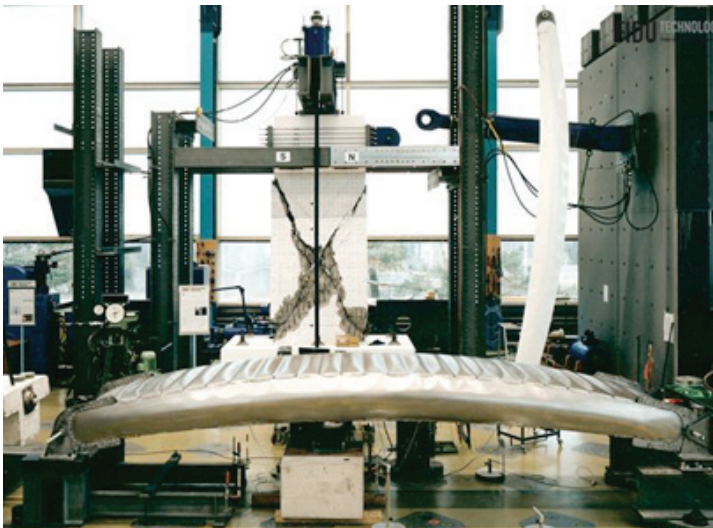
FIDU-Bridge, 2007, preparation for the static load test, external dimensions: 6m x 1,5m, weight: 174 kg, load: 1850kg
