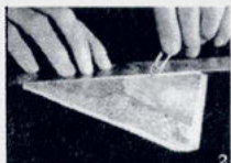
SCORING OF MARGINS of colored face of map segment with sharp ball point facilitates folding of paper (right).
