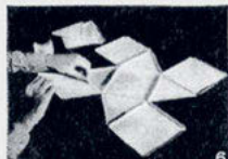
EQUATORIAL SQUARES are then joined to polar square—straight assembly, keep letters roughly matching.
