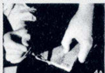
HOUSEHOLD PASTE on margins is best means for fastening flaps. It should be spread thinly to avoid warping.
