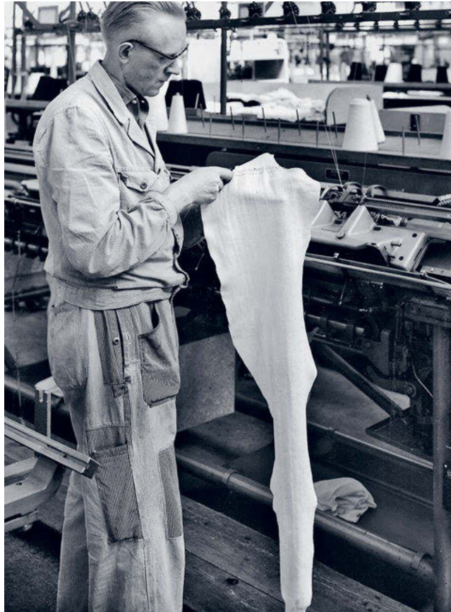
Fig. 2: A machine operator at Hanro checks a knitted fabric intended for a pair of ski underpants; a flat knitting machine is visible in the background. The photograph was taken in 1958.
